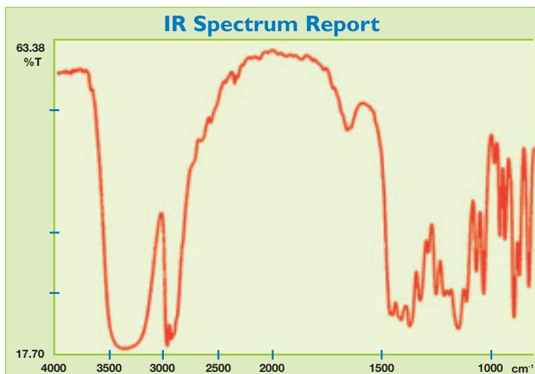
**IR spectrum of a polyhydric alcohol, the primary component of AMTECH's polymer activator**
