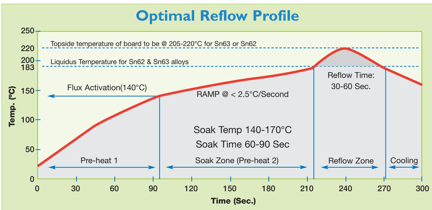
Many reflow machines available today include an on-board profiler, even some of the smaller, less expensive, bench-top ovens. If the oven being used is not equipped with a profiler, after market temperature profilers are available.
